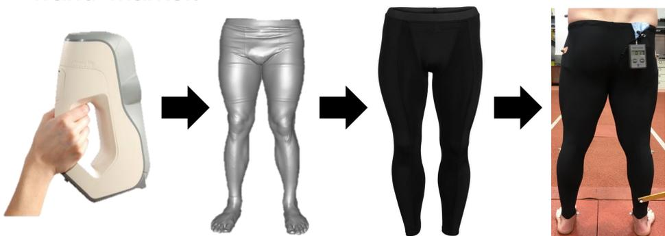
Figure 1. Schematic of the methodology beginning with a 3D scan, manufacturing the garments using the 3D model and subsequent assessment of pressure.
